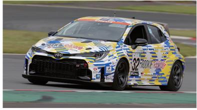
GR Corolla fueled by liquid hydrogen
