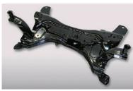
Suspension member made with Kobe Steel's Kobenable A suspension lower arm made by Tokyo Steel from mass balance methodology)
